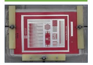
Developing new Magnesium alloy photoengraving plate for Graphic Arts application that increases life of dies and makes it more competitive vs. copper or brass
