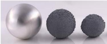
**Material for Dissolvable Frac Plugs used in Plug and Perf operations**
