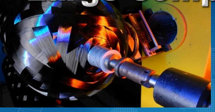
Luxfer's composite Type 3 (aluminumlined) alternative fuel (AF) cylinders are used to contain compressed natural gas (CNG) for buses and medium duty trucks.
