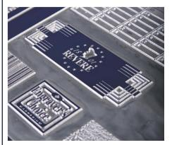
Includes magnesium, copper and brass plates for photo-engraving, embossing and foil stamping.
